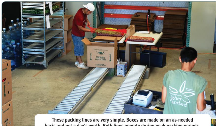
These packing lines are very simple. Boxes are made on an as-needed basis and not a day's worth. Both lines operate during peak packing periods.
